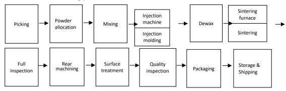
D. Manufacturing process for hinge parts (milling parts)
